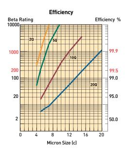
Notes: Multipass test run @ 80 gpm to 50 psid terminal - 5 mg/l BUGL.
