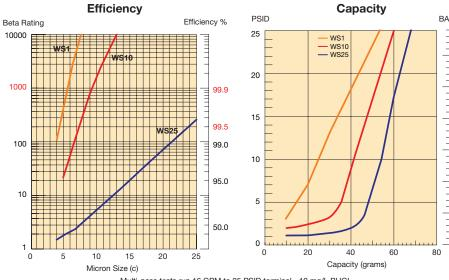
Multi-pass tests run 16 GPM to 25 PSID terminal - 10 mg/L BUGL
