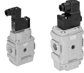
Remotely operated dump valves automatically shut off upstream pressure and exhaust the downstream pressure when the pilot pressure is released.
