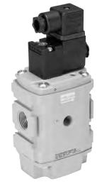
Parker Global Series Combined Soft Start / Dump Valves. provide for the safe introduction of pressure to machines or systems. Soft Start / Dump Valves when set, allow the pressure to gradually build to the set point before fully opening to deliver full flow at line pressure.
