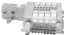
The Isys Micro is designed with an innovative back-to-back valve mounting style where 4 valves are assembled on a 42mm wide manifold, producing an equivalent 10.5mm valve width.
