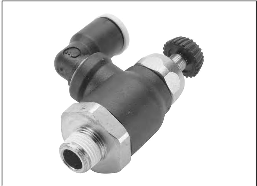
Flow control regulators with “swivel outlet” are especially designed to allow a vertical or angled tube exit where access is restricted. The swivel outlet comes with instant push-in connection to ease installation. Flow control regulators with swivel outlet are available in meter out and meter in versions.
