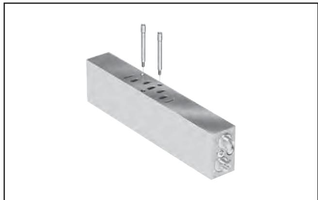
*A Sandwich Flow Control and Common Port Sandwich Regulator may be sandwiched together on a manifold or subbase. The Sandwich Flow Control MUST be located between the manifold/subbase and the Common Port Sandwich Regulator.*
